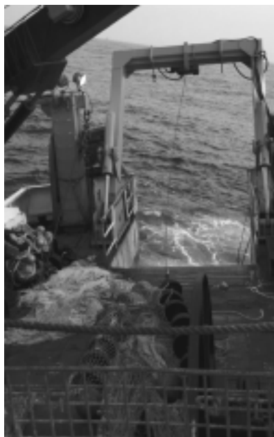
Trawl Ramp and Gantry
