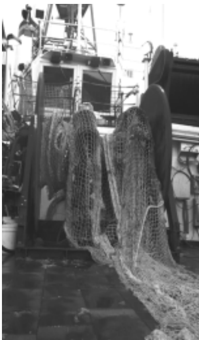
Winch Control Room above Net Reel
