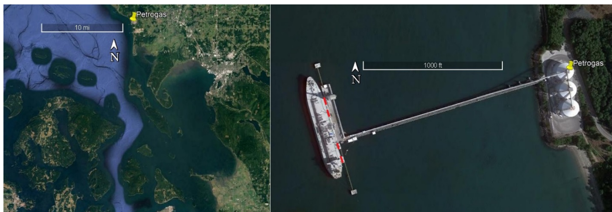
Figure 1. Google satellite photographs of the Petrogas Pacific LLC project site in Whatcom County, Washington. The left image shows the location of the project site relative to Bellingham, Washington, which is visible to the southeast of the site. The right image shows the applicant’s pier. The four breasting dolphins to be replaced are identified in red. The piles that would be repaired are scattered under the entire mooring structure.
