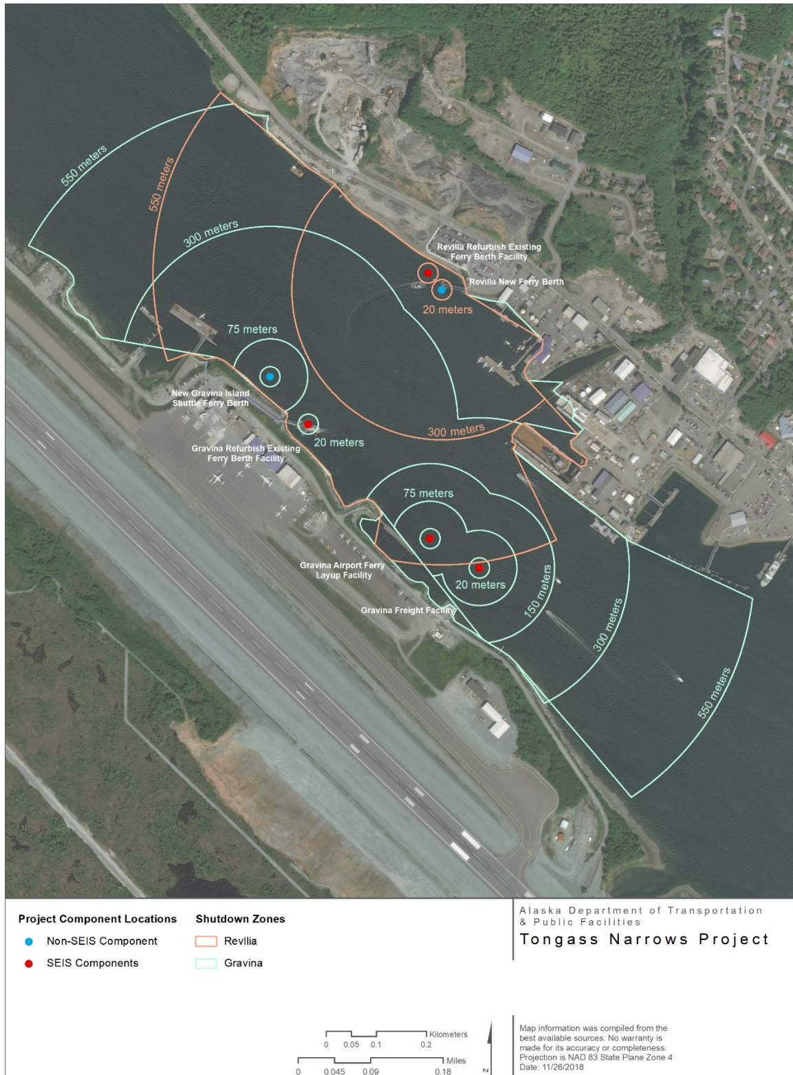
Figure 9. Level A shutdown zones for pile installation and removal activities at the Tongass Narrows Project (figure prepared by HDR for this opinion).
