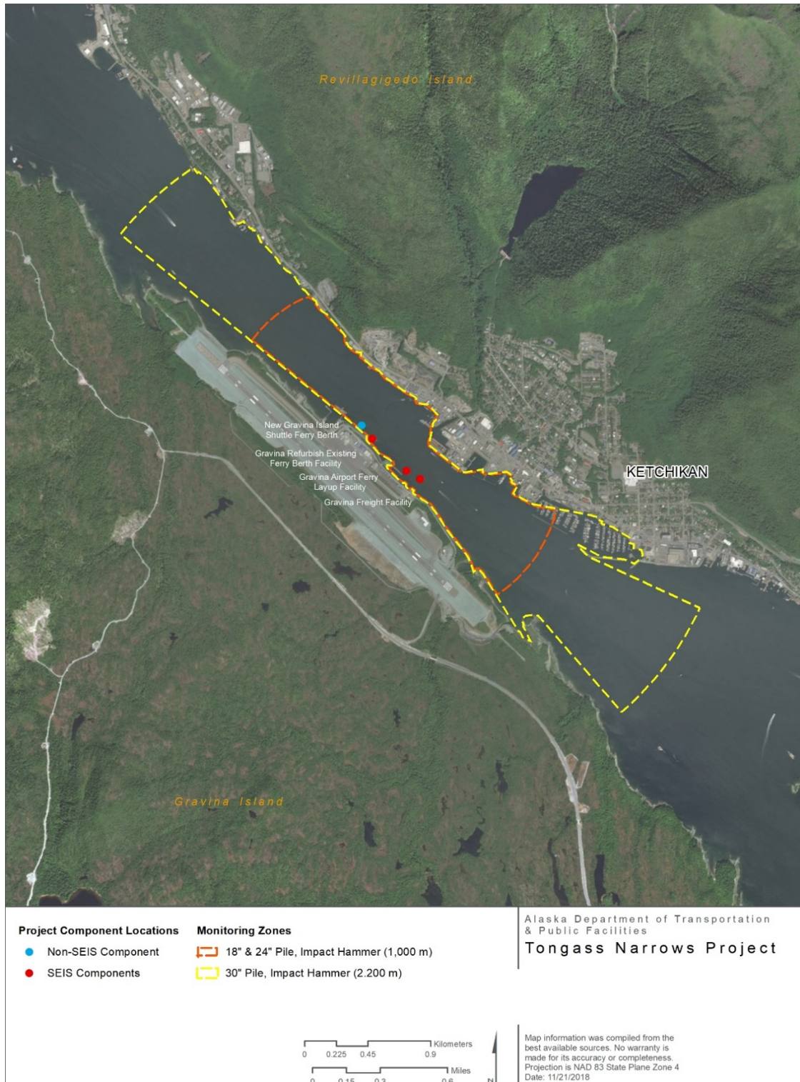
Figure 10. Level B monitoring zones for impact installation of 18-inch, 24-inch, and 30-inch diameter round steel piles at Tongass Narrows Project locations on Gravina Island (figure prepared by HDR for this opinion).
