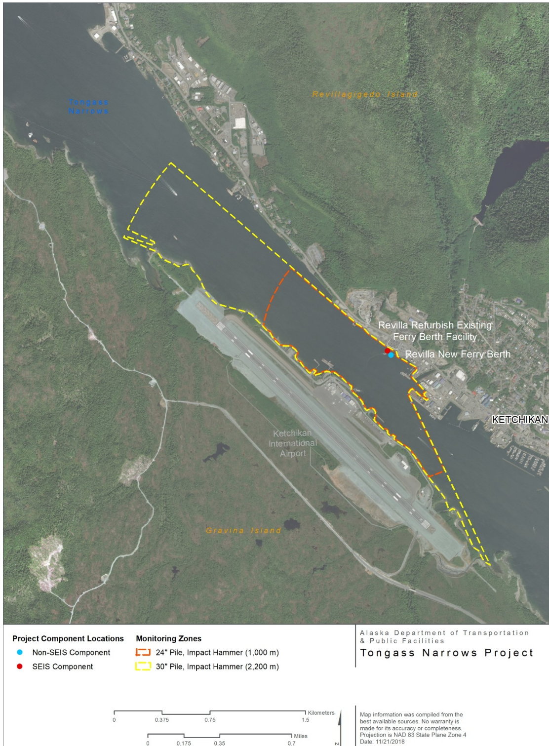
Figure 12. Level B monitoring zones for impact installation of 24- and 30-inch diameter round steel piles at Tongass Narrows Project locations on Revillagigedo Island (figure prepared by HDR for this opinion).
