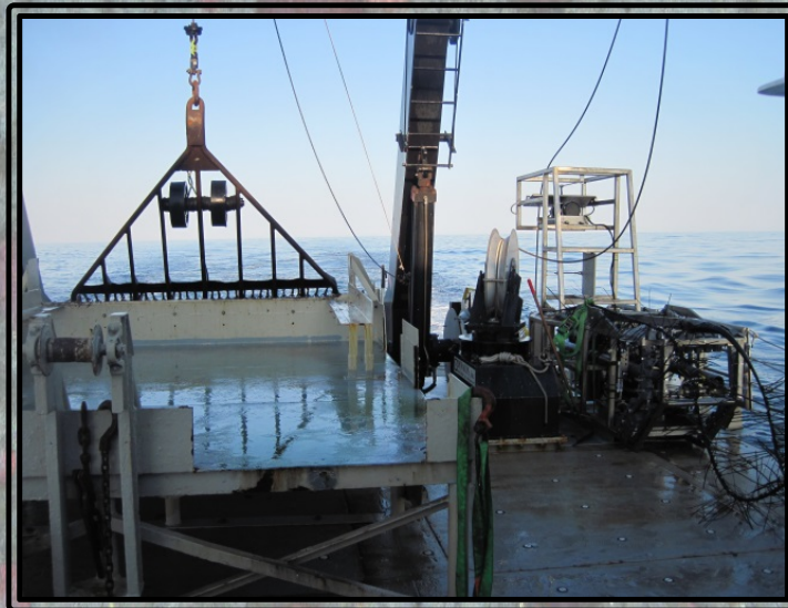
A view of both the dredge and HabCam on the back deck
