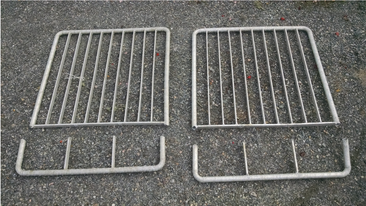
Figure 7. Both broken TEDs removed from the extension pieces
