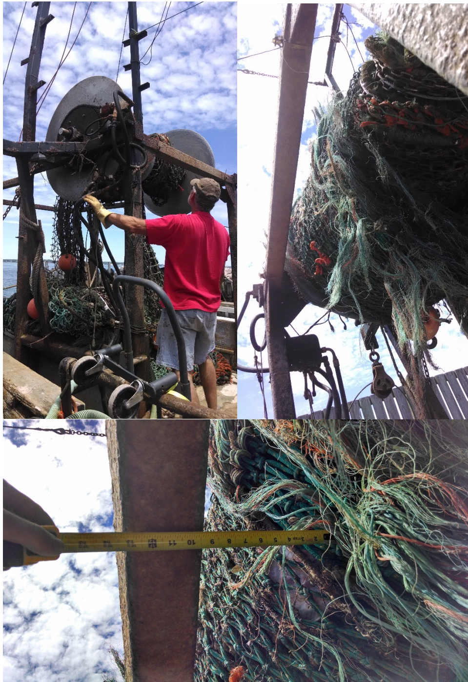
Figure 2. The net reel aboard the FV Elizabeth J showing the horizontal cross bar forward of the reel preventing the installation of the TED
