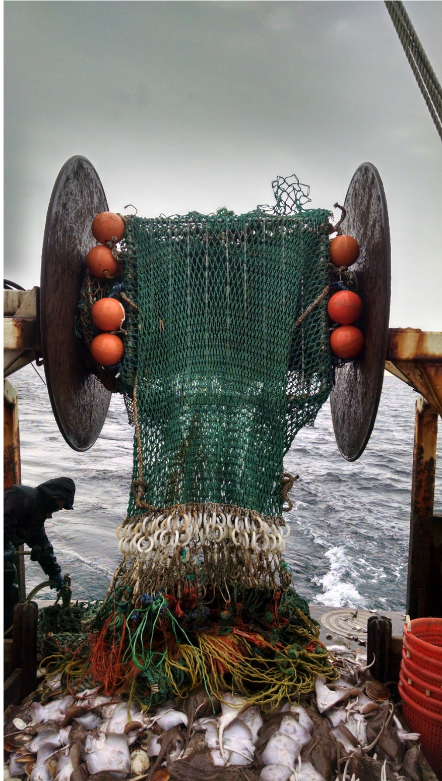
Figure 6. TED on net reel after breaking horizontally above windows aboard the FV Two Anns
