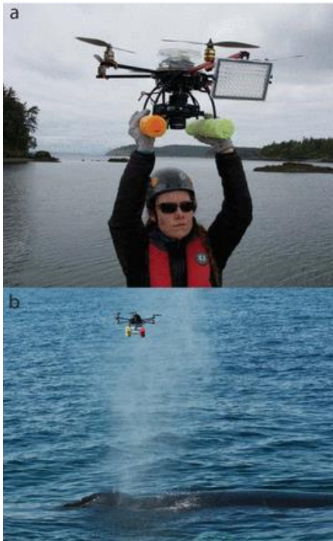
Figure 6. Example of a vertical take-off and landing unmanned aircraft system, the APH-22, used for breath sampling under Permit Nos. 19091 and 17355.
