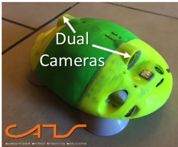
Figure 12. Example of a suction-cup tag by Customized Animal Tracking Solutions with two cameras, accelerometers, global positioning system, temperature and depth sensors, and a very high frequency transmitter from File No. 20430.
