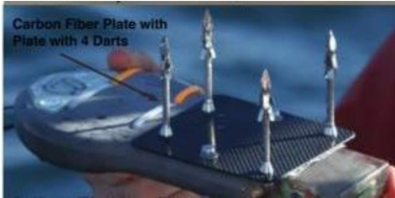
Figure 16. Example of a dive-location dart/barb tag with a TDR 10-F (Wildlife Computers) Very High Frequency transmitter and floatation from File No. 20430.
