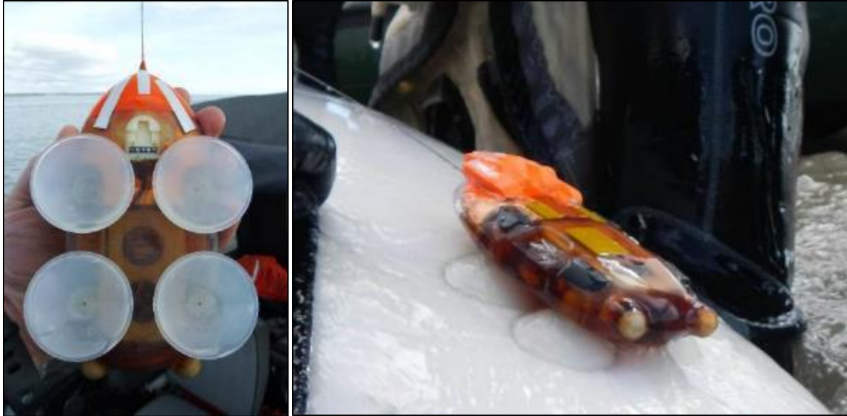
Figure 11. Example of a suction-cup tag with an acoustic recording instruments in hand (left) and attached to a beluga whale (right) from File No. 20556.
