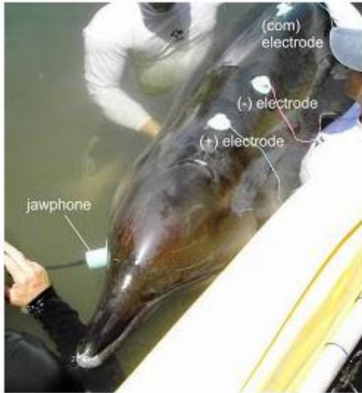
Figure 9. The typical three-sensor configuration and jawphone for Auditory Evoked Potential testing (from File No. 21026).
