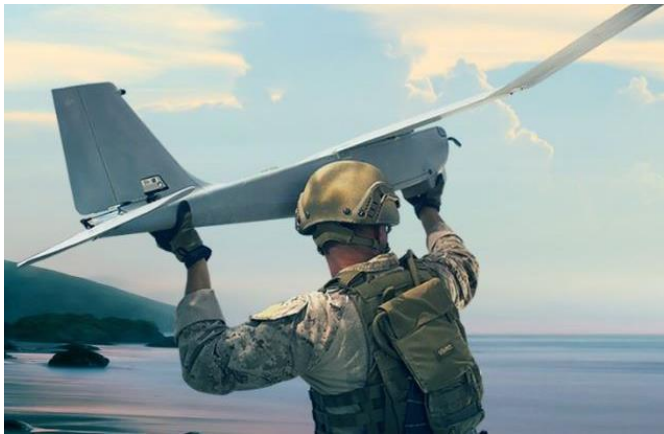
Figure 4. Example of a larger fixed-wing unmanned aircraft system, the Puma AE by AeroVironment.
