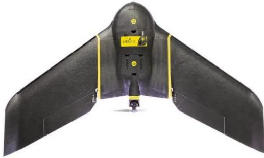
Figure 3. Example of a small and lightweight fixed-wing unmanned aircraft system, the eBee Plus by senseFly.
