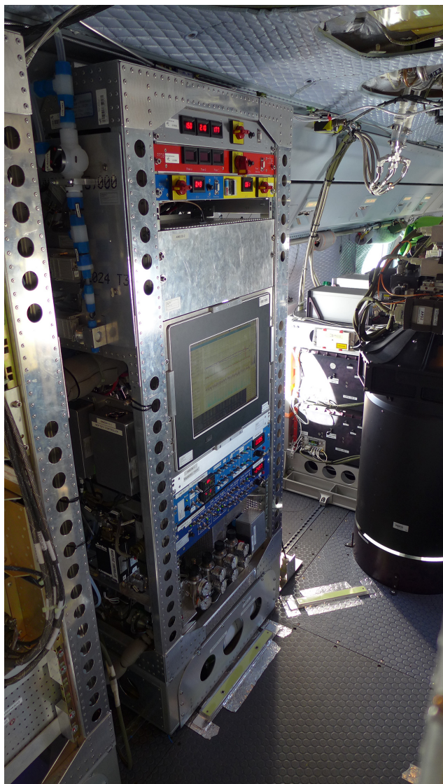
Figure 1. Front view of instrument rack in AIMS-H 2 O configuration integrated in a HALO standard rack. The inlet line is connected to a trace gas inlet (TGI) mounted at the top fuselage of the aircraft.
