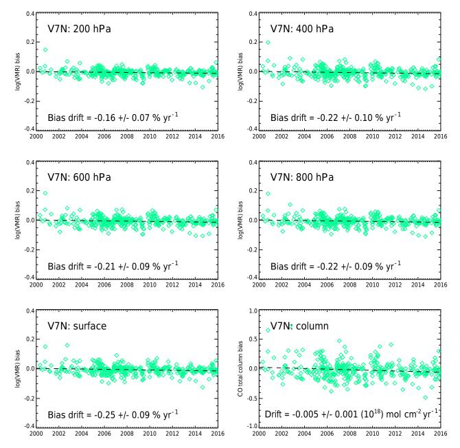
Figure 14. Retrieval bias drift for V7 NIR-only products based on the NOAA flask measurements. See caption to Fig. 11.
