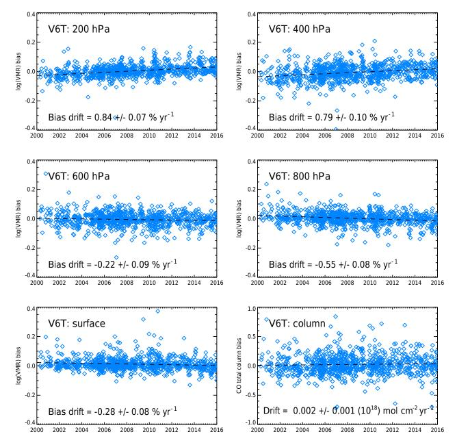
Figure 11. Retrieval bias drift for V6 TIR-only products based on the NOAA flask measurements. CO total column bias values are given in units of  $10^{18}$  molec cm<sup>-2</sup>.
