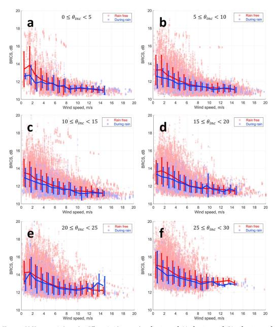
**Figure 3.** BRCS versus wind speed at different incidence angles:  $0^{\circ} \le \theta_{\text{inc}} < 5^{\circ}$  (a),  $5^{\circ} \le \theta_{\text{inc}} < 10^{\circ}$  (b),  $10^{\circ} \le \theta_{\text{inc}} < 15^{\circ}$  (c),  $15^{\circ} \le \theta_{\text{inc}} < 20^{\circ}$  (d),  $20^{\circ} \le \theta_{\text{inc}} < 25^{\circ}$  (e), and  $25^{\circ} \le \theta_{\text{inc}} < 30^{\circ}$  (f). BRCS = bistatic radar cross section.
