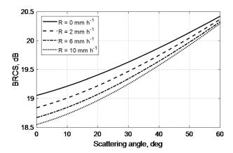
**Figure 5.** BRCS  $\sigma^0$  versus the scattering angle for  $U_{10}=3$  m/s at different rain rates R. BRCS = bistatic radar cross section.
