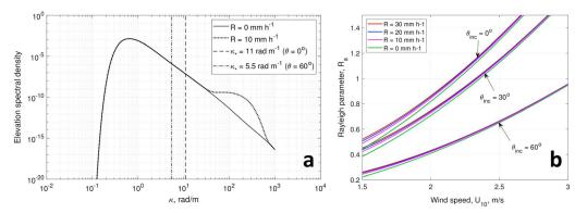
**Figure 1.** Wave elevation spectrum (a) at wind speed 3 m/s without rain and modified by rain (rain rate R=10 mm/hr) along with the  $k_*$  for incidence angles of 0° and 60° shown with vertical dashed and dash-dotted lines and surface roughness Rayleigh parameter  $R_a$  (b) versus wind speed for a range of rain rates and for three incidence angles  $\theta_{\rm inc}$ .
