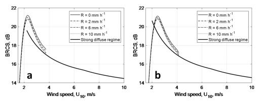
**Figure 6.** BRCS  $\sigma^0$  versus wind speed for scattering angles of  $0^{\circ}$  (a) and  $30^{\circ}$  (b) at different rain rates *R*. BRCS = bistatic radar cross section.
