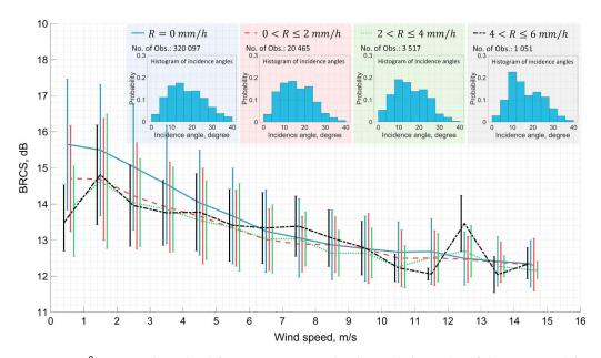
**Figure 2.** BRCS  $\sigma^0$  versus wind speed at different rain rates R (mm/hr) along with the number of observations and the histogram of incidence angles for the measurements in each rain rate bin. BRCS = bistatic radar cross section.
