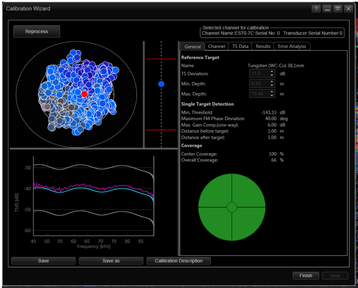
Figure 18. Screenshot of EK 80 Calibration Wizard. General results for 70 kHz calibration at 1.024 ms in FM mode.
