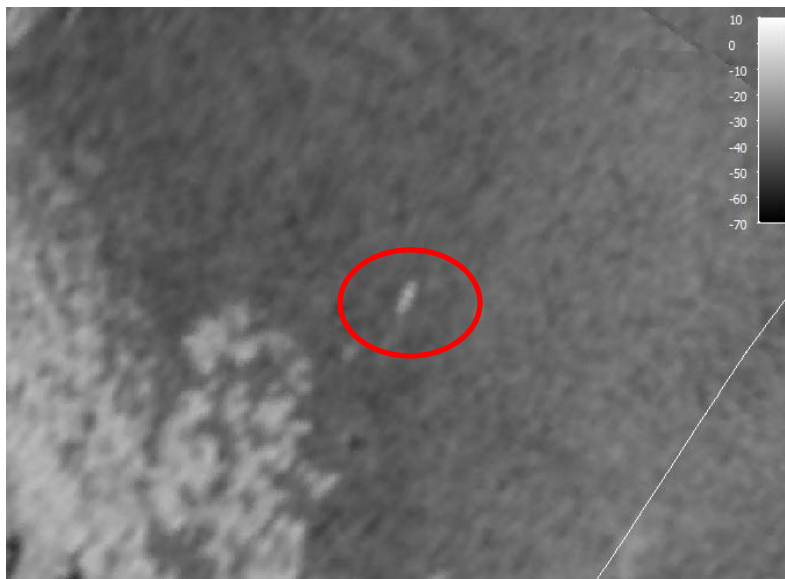
Figure 16. Seafloor backscatter mosaic (obtained from Line # 30) showing a distinct target (highlighted in red circle).
