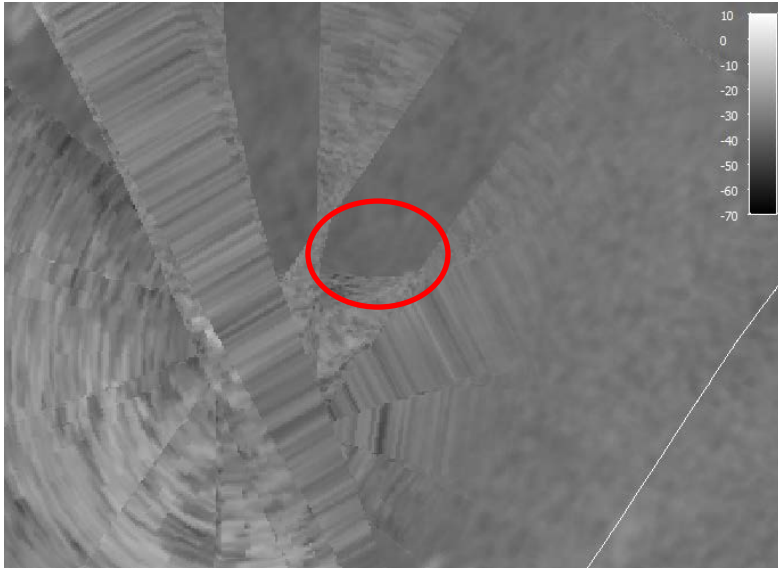
Figure 17. Seafloor backscatter mosaic after combining the data obtained with EM 302 run in 3D scanning mode (Line # 21)
