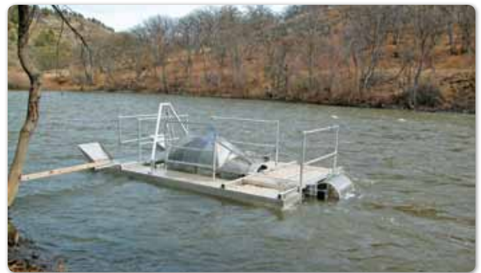
Exhibit 22: Rotary Screw Trap Used to Monitor the Abundance of Outmigrant Juvenile Salmonids on the Klamath River Near Bogus Creek. Photo courtesy of USFWS.
