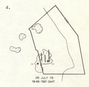
Figure 1. PPI echo envelopes (hatched areas) and approximate flight tracks of chaff-dispersing aircraft (broad, vertical lines) within R2902. Turret locations are denoted by a •; the nearby numbers are the maximum observed turret heights in km.
