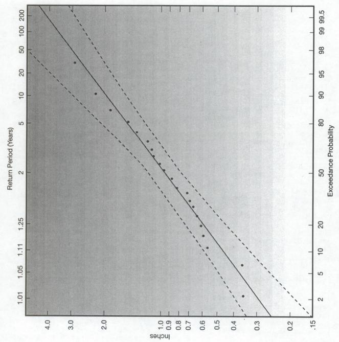
Figure 21. Log Pearson Type III fit to annual maximum daily precipitation totals for Jackass Flat, (4JA), 1976 through 1995. Dashed lines enclose 95% confidence limits.
