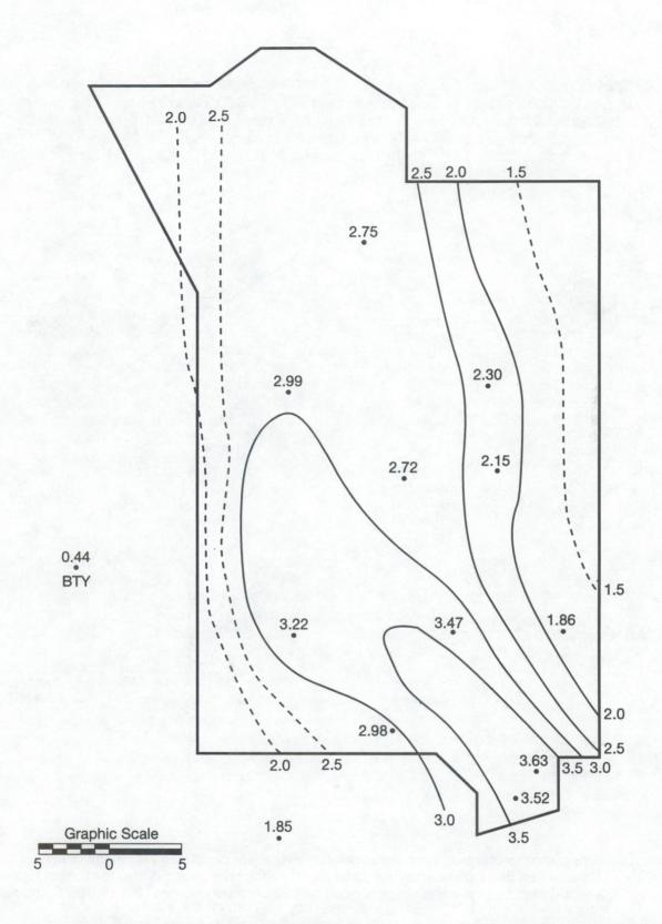
Figure 10a. Isopluvial analysis of the daily precipitation totals, in inches, for the Nevada Test Site for August 18, 1983. Dashed contours are estimated positions.
