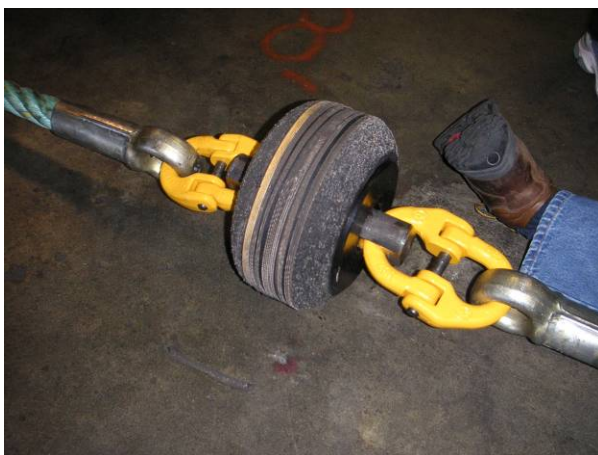
10 inch elevating bobbin connected to 2 inch (52mm) combination wire with hammerlocks (coupling links)
