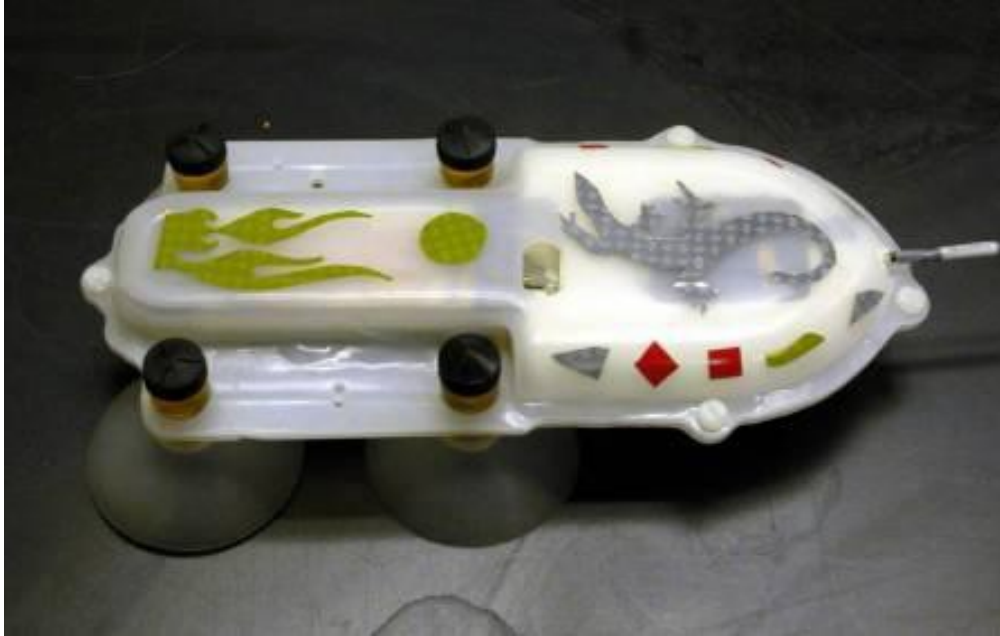
Figure 7. Example of a Digital Acoustic Recording Tag (DTAG) in casing with suction-cups.
