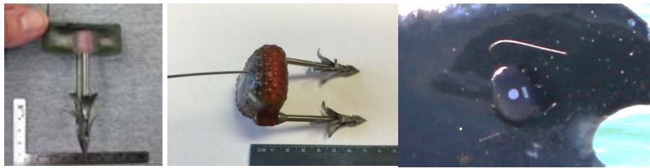
Figure 11. Example of a Wildlife Computers Mk 10-A depth transmitting LIMPET tag with two titanium dart/barbs that penetrate 6.5 centimeters (left), Wildlife Computers SPOT tag with two dart/barbs that penetrate 6.5 centimeters (center), and Wildlife Computers LIMPET-F GPS Fastloc location-dive tag deployed on a humpback whale under Permit No. 16239 (right).
