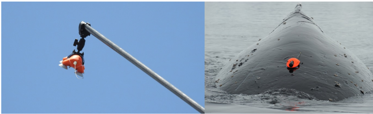
Figure 8. Example of a customized animal tracking solutions suction-cup tag attached to a pole and attached to an animal via suction-cups.
