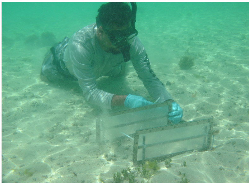
Figure 6. Image of NOAA scientist installing duplicate PEDs in the waters around Cocos Island, Guam.
