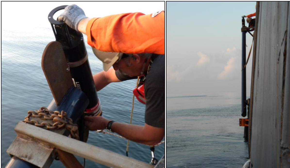
Figure 2-4. This Sequoia Scientific LISST 100X (left) was deployed during Deepwater Horizon water quality studies to observe particle size distribution and volume concentration. While on station, a short time series of surface data was collected using a boom mounted on the side of the RV Ocean Veritas (right). A second short time series was collected while underway to the next station. (Photos courtesy of Mark Bushnell)
