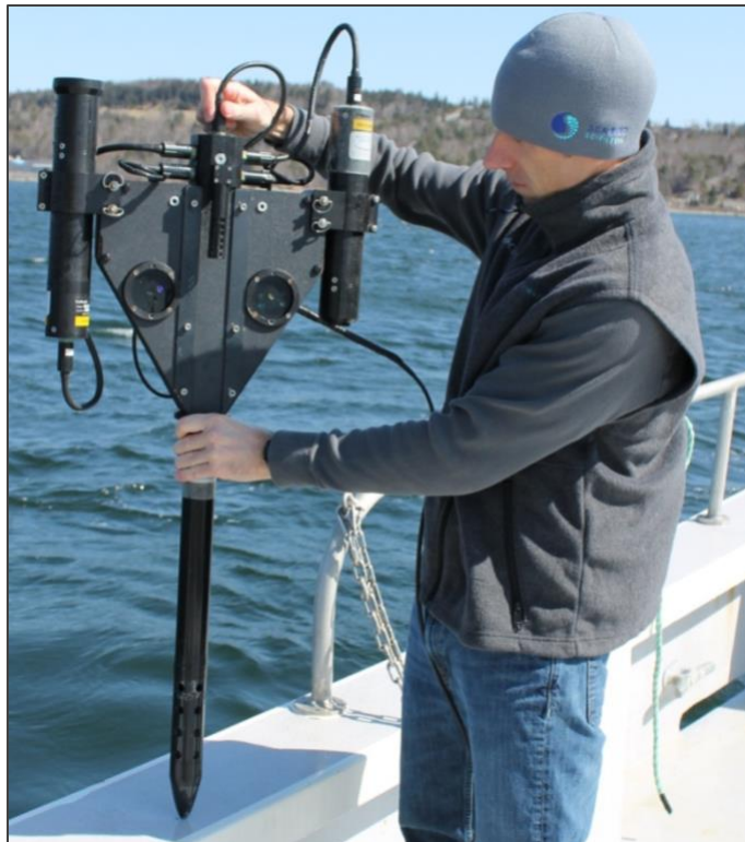
Figure 2-5. Various optical instruments (including multi-spectral downwelling irradiance and upwelling radiance) are installed and deployed aboard this Satlantic Profiler II, which can free-fall through the water column or be lowered using a tether. (Photo courtesy of Todd Yeadon/Sea-Bird Scientific)
