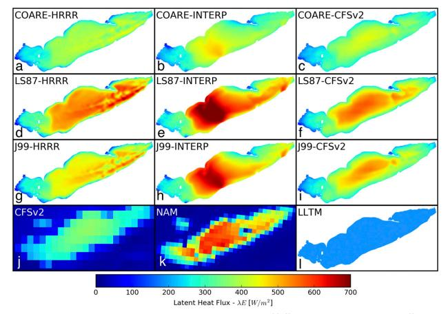
FIG. 5. Snapshots of the peak modeled latent heat flux  $\lambda E$  at 1200 UTC 18 Nov 2014. (a)—(i) Results from FVCOM. Results from (j) CFSv2, (k) NAM, and (l) LLTM. Note that the LLTM result in (l) shows the daily and lakewide average values.
