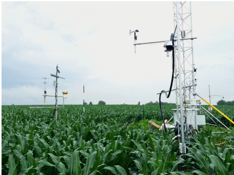
8 9 Figure 1: The relaxed eddy accumulation (left tower) and flux gradient (right tower) measurement systems 10 were located 5 m apart in the center of the study plot.
