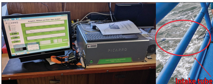
Figure 5.1. CRDS-Picarro placement inside of the dry-lab of the R/V Brooks McCall (left); and sample intake tube location on the forward lower deck, starboard side of the vessel (right).
