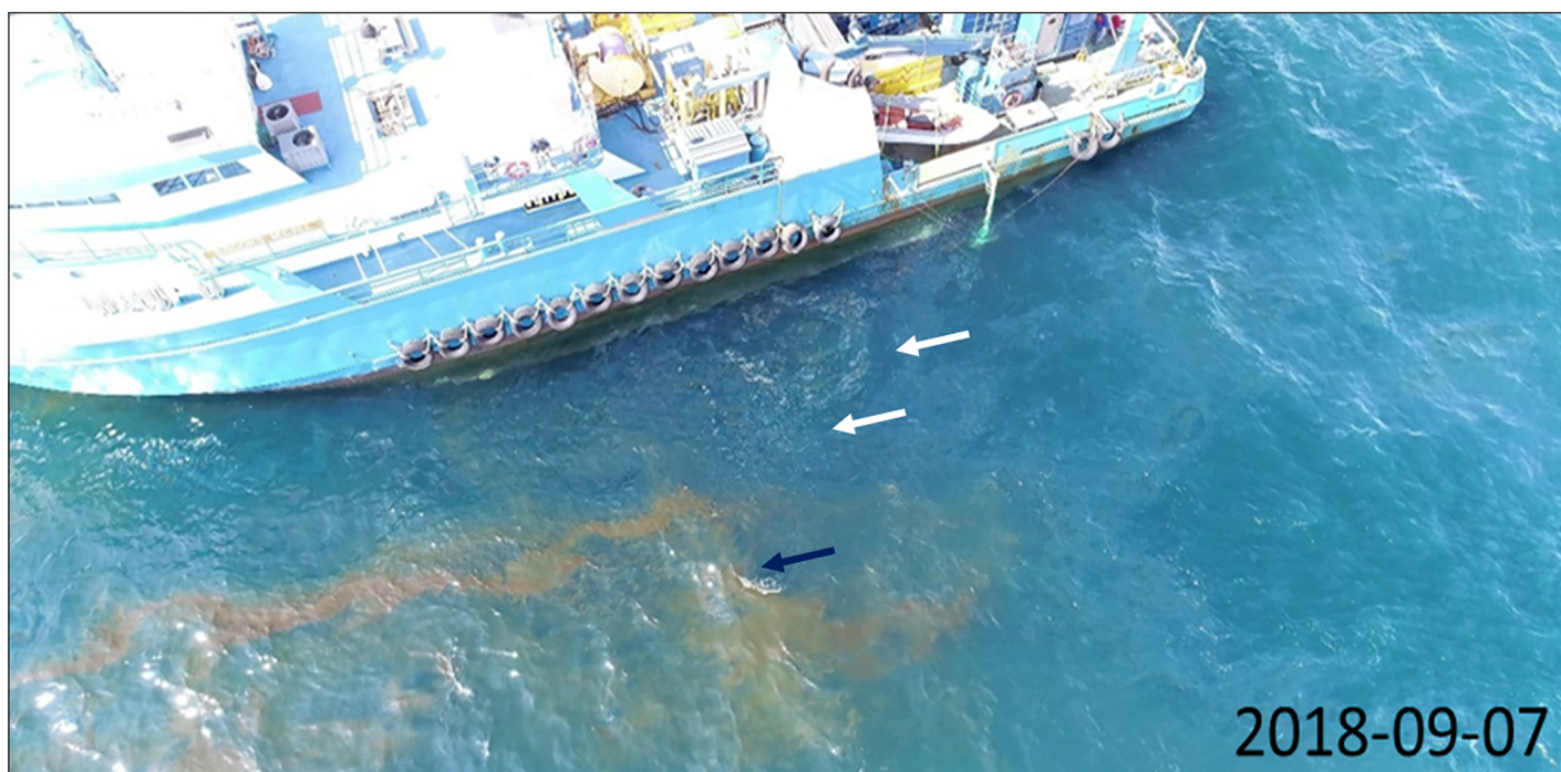
Figure 3.19. Drone image of R/V Brooks McCall with rising gas plume and oil at the surface. Surfacing gas bubbles identified by white arrows, surfacing oil slick identified by blue arrow.
