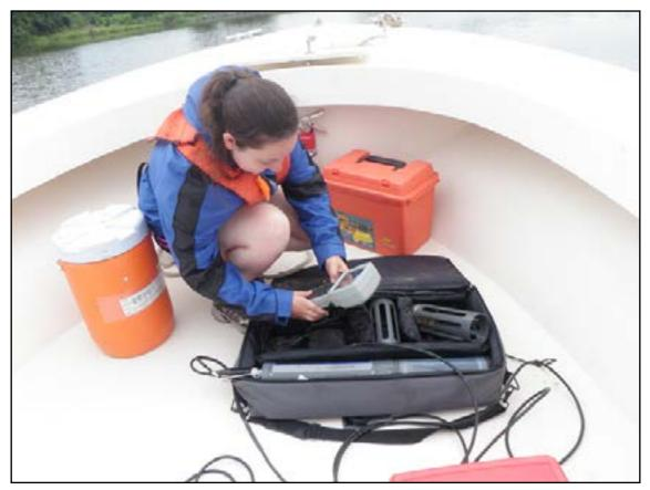
**Image WQ2.** A YSI data sonde<sup>®</sup> (YSI, Inc., Yellow Springs, OH) is being assembled prior to measuring water quality parameters such as dissolved oxygen, temperature, salinity, and turbidity in the Tred Avon River ecological assessment.
