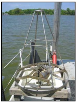
**Image BH1.** A Young-modified Van Veen grab is used to collect sediments for laboratory analyses.
