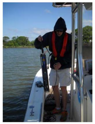
**Image WQ3.** A YSI data sonde<sup>®</sup> (YSI, Inc., Yellow Springs, OH) is used to measure water quality parameters in the Tred Avon ecological assessment.
