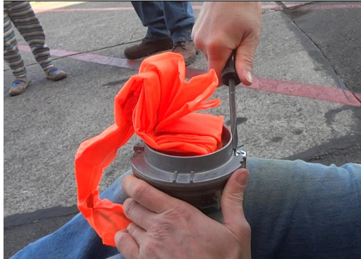
Figure 7b. Use a small thin standard screwdriver to pry up the silver bars on either side of the top component.
