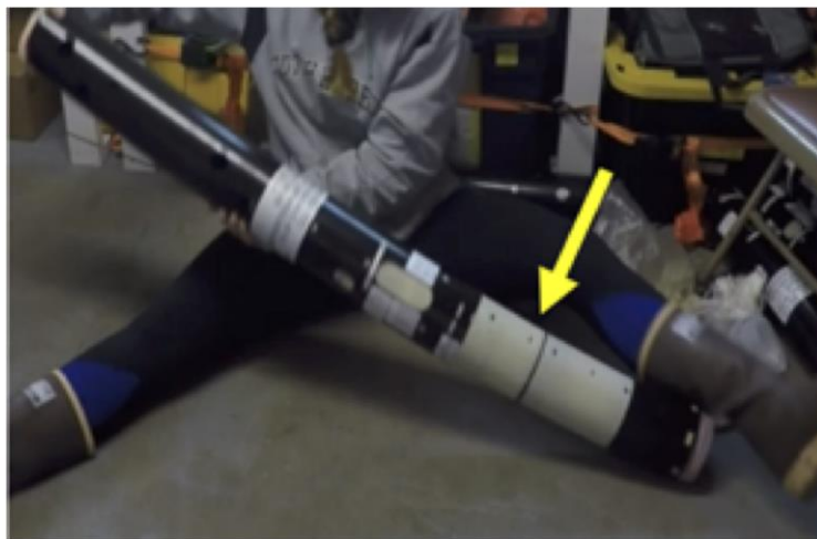
Figure 2a. Carefully pour out the sonobuoy until the top of the third component is accessible (yellow arrow), trying to keep everything else intact. Note: this is a different type of sonobuoy, but the plastic housing of the inner components look similar.
