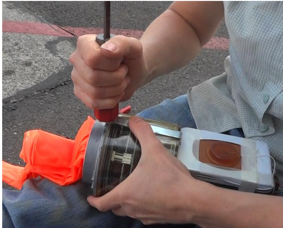
Figure 7h. After ensuring that the display battery now works (by hitting the Verify button), replace the metal bars on the side of the housing. Place one end in the groove, then using the end of the screwdriver, tap the other end until the bar snaps in place. This may take some force.
