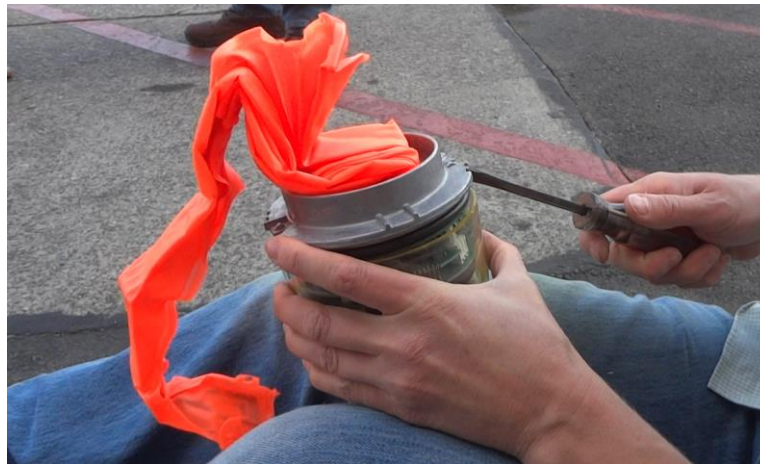
Figure 7c. Use the screwdriver to pry the lid off the top of the component.
