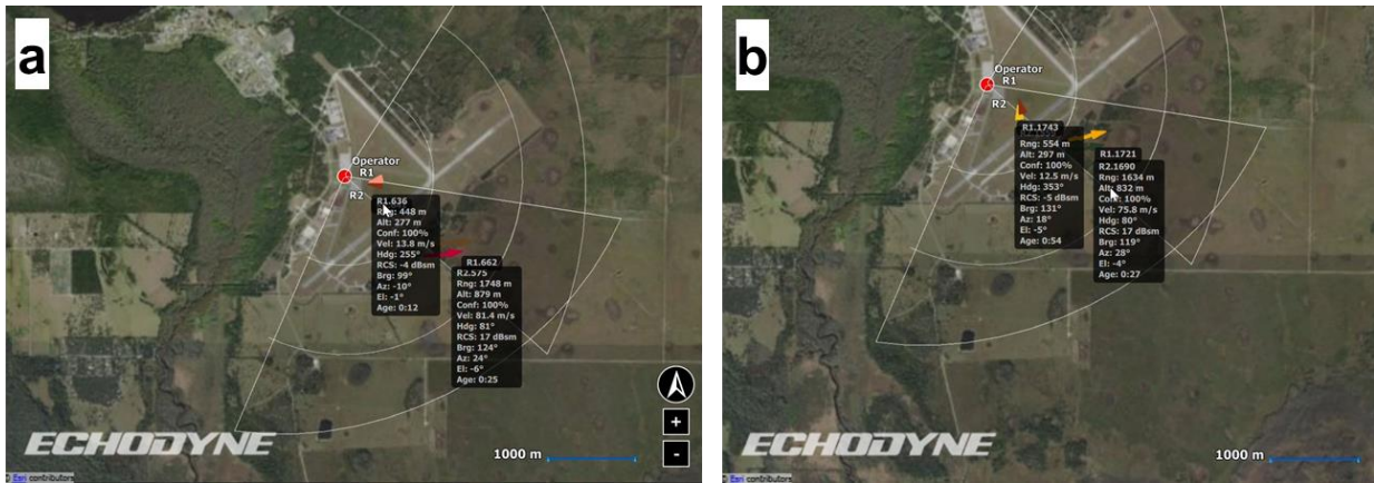
Figure 12: Echodyne software detecting the BST S2 (left target) and NOAA Twin Otter Aircraft (right target). Image taken at 14:08 UTC (panel a) and 14:12 UTC (panel b) 5 March 2019.
