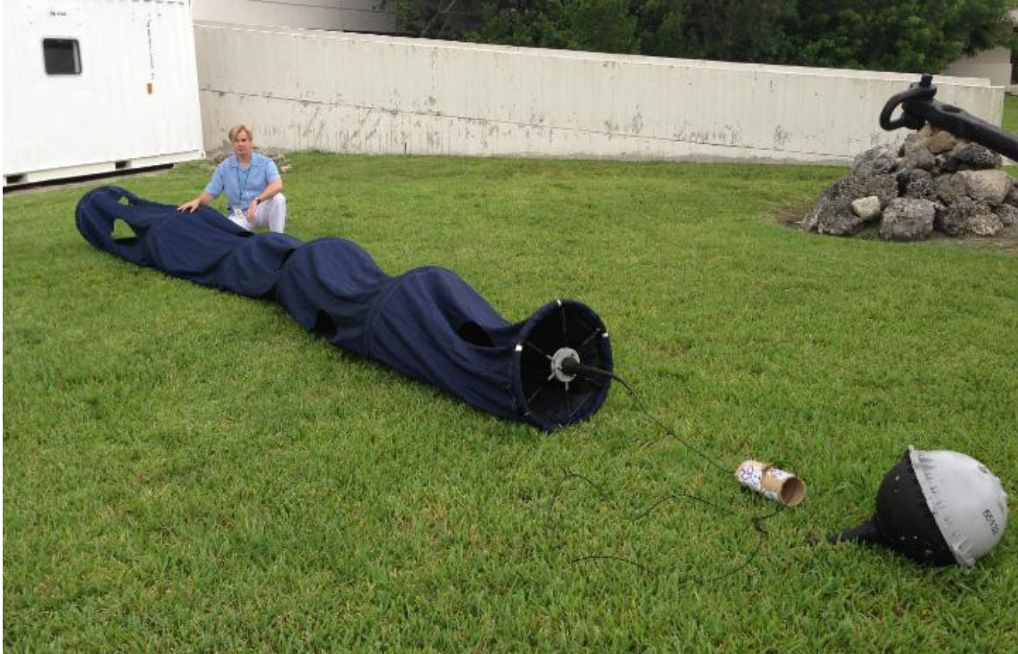
Figure 1. A Surface Velocity Program (SVP) drifter, with author Rick Lumpkin for scale reference. At left is the holey-sock drogue, centered at a depth of 15 m when the instrument is deployed. The drogue is attached to the surface float ( bottom right ) by a tether, much of which is bound by paper tape inside a cardboard tube for ease of deployment.
