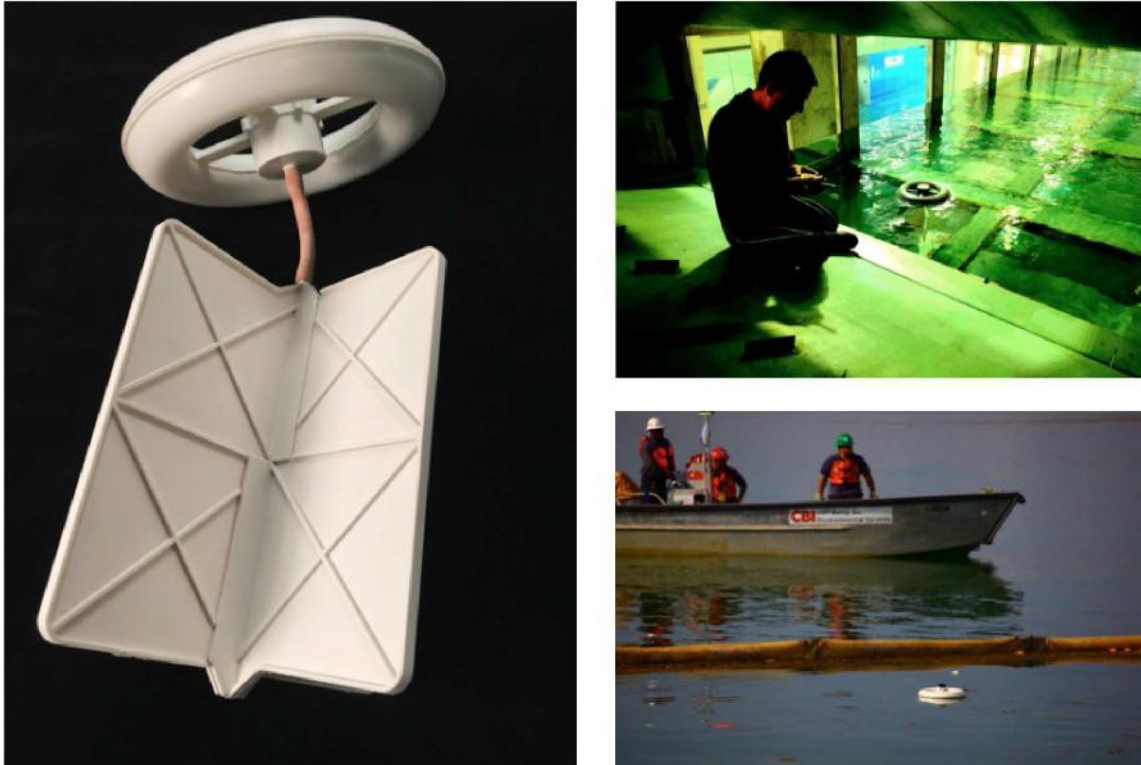
Figure 3. (a) A biodegradable Lagrangian Submesoscale Experiment (LASER) drifter. (b) LASER drifter testing in the University of Miami wave tank. (c) A LASER drifter being used during an oil spill exercise. Images provided by the Consortium for Advanced Research on Transport of Hydrocarbon in the Environment ( http://carthe.org ).
