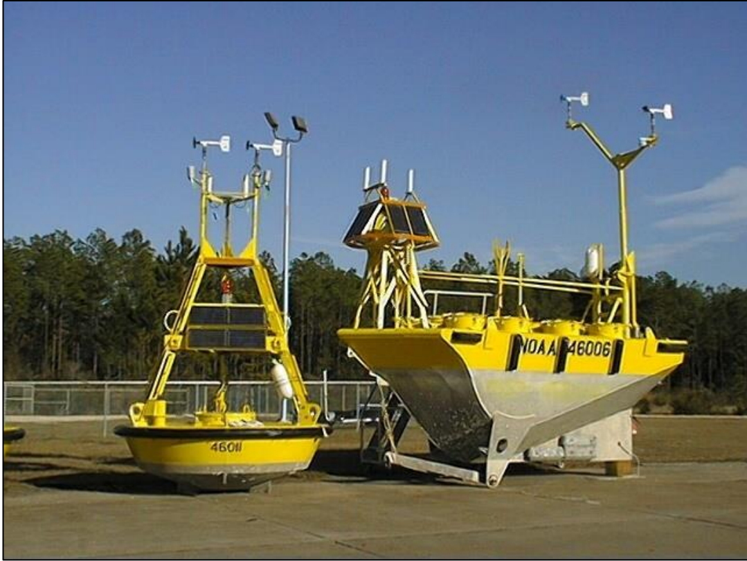
Figure 2-1. NDBC 3-m discus buoy (left); NDBC 6-m NOMAD buoy (right). (Photo courtesy of Richard Bouchard/NDBC)
