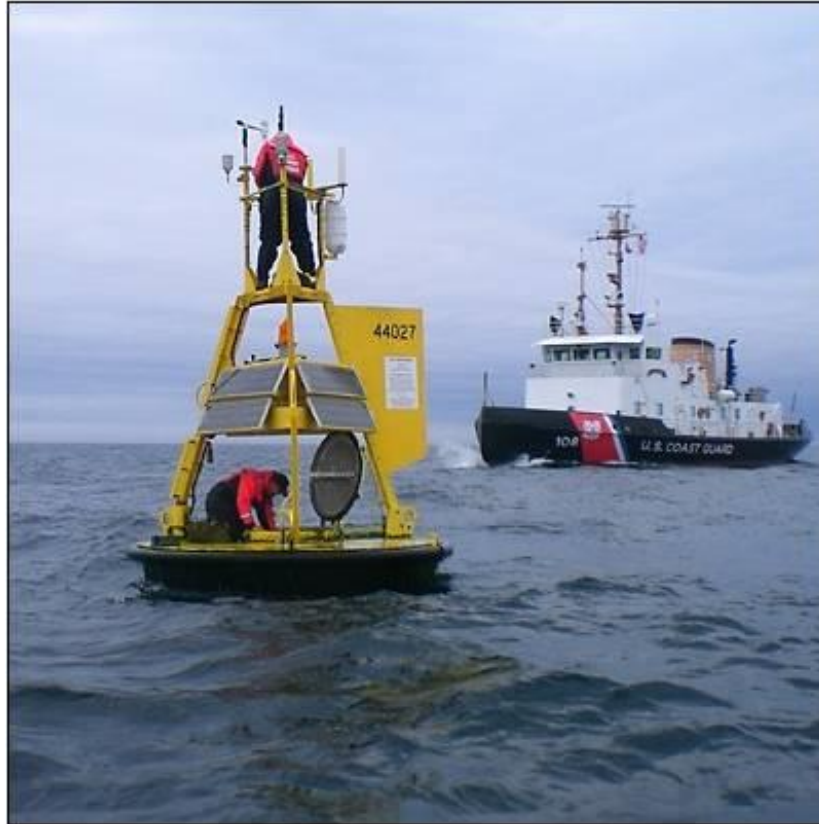
Figure 2-2. NDBC 3-m disc buoy being serviced at sea from U.S. Coast Guard vessel. (Photo courtesy of Richard Bouchard/NDBC)
