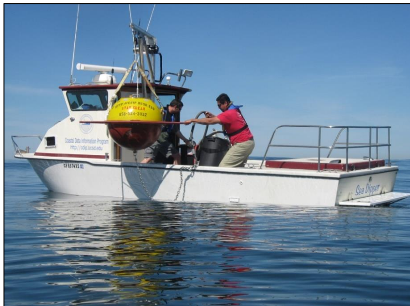
Figure 2-3. CDIP personnel deploy a Datawell directional Waverider. As of 2019, the CDIP network is composed of approximately 65 wave observation sites. (Photo courtesy of SIO/CDIP)
