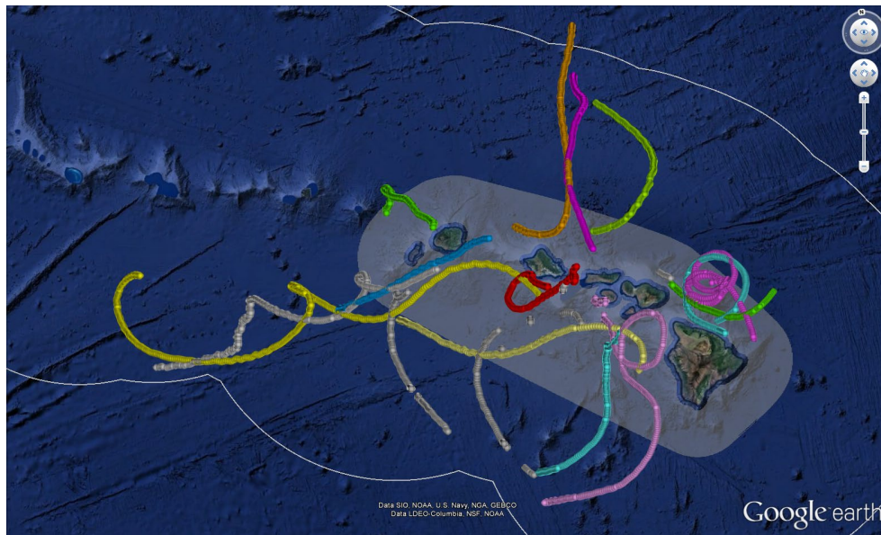
Figure 4. DASBR tracks during HICEAS 2017. Tracks in gray halted transmission prematurely, and therefore were unable to be retrieved. The Hawaii EEZ boundary is shown by the gray line and the main Hawaiian Islands Focus Area is shaded gray.
