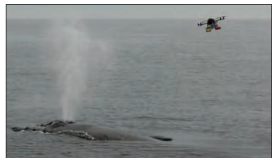
Sampling whale's breath using an unmanned hexacopter.
