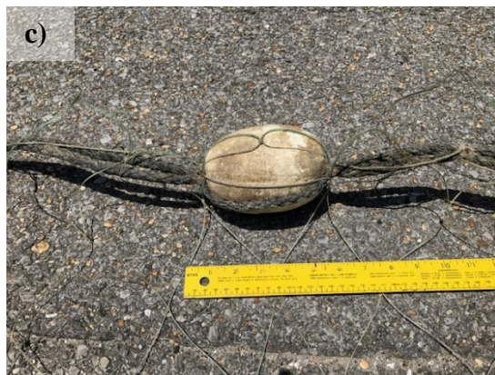
Figure 3. Characteristics of the gillnet, a) the gillnet had a double leadline with a 3/8 inch leadcore rope and a twisted poly rope with three (4.5 oz. each) lead weights per yard, b) gillnet stretched mesh was 9 inches with ~1.1 mm diameter; the gillnet was 15.5 meshes deep, c) top of the gillnet had 5 inch floats placed 6 3/4 ft. apart.
