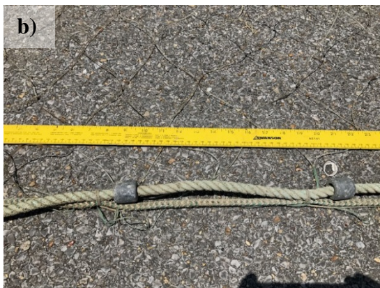
Figure 3. Characteristics of the gillnet, a) the gillnet had a double leadline with a 3/8 inch leadcore rope and a twisted poly rope with three (4.5 oz. each) lead weights per yard, b) gillnet stretched mesh was 9 inches with ~1.1 mm diameter; the gillnet was 15.5 meshes deep, c) top of the gillnet had 5 inch floats placed 6 3/4 ft. apart.
