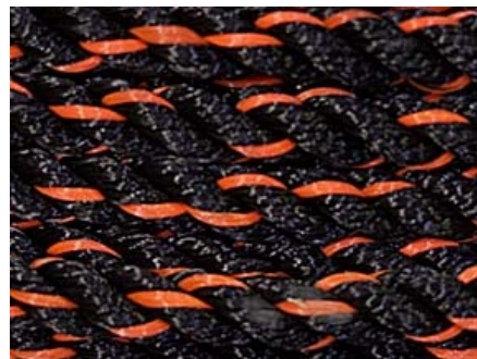
Figure 2.10.1. Example of a color tracer line (orange) woven along the entire length of a black trap line. In the image, the trap line is coiled.
