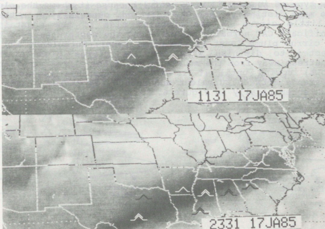
Figure 4. GOES 6.7 micron water vapor images showing an episode of darkening with time over a 12 hour period. Turbulence reports within 3 hours of each image are superimposed.
