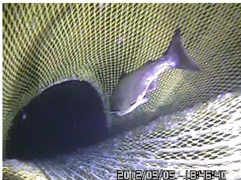
Figure 23. Upper escapement panel and upper escapement portal (port camera)
