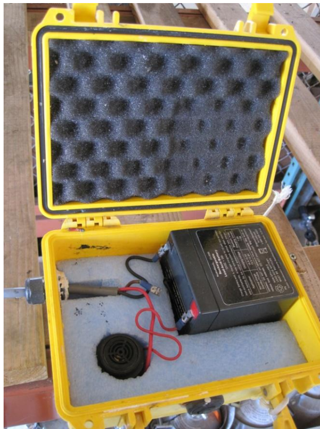
Figure 45. Receiving end of the signal with the battery, speaker, and electrical connections in a pelican case housing.
