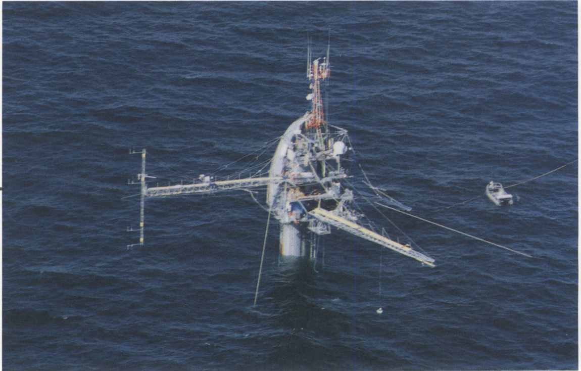
Fig. 7. Photo of FLIP taken from a blimp during COPE. The 5-mm radiometer was installed on the port boom in the left side of the figure.
