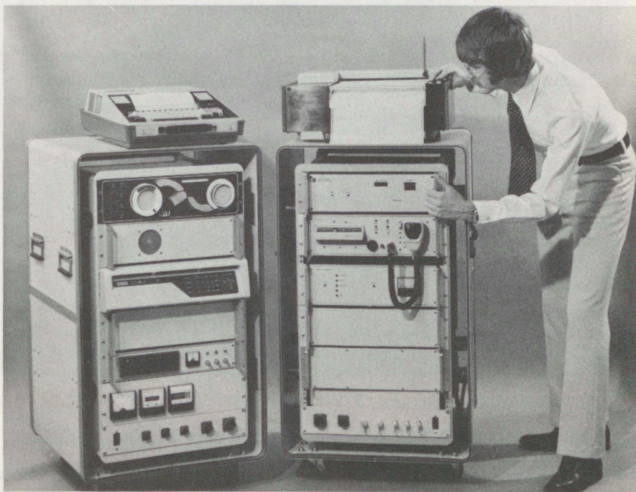
Figure 9. Current-sensing-radar components mounted in their fiberglass cases for field use.
