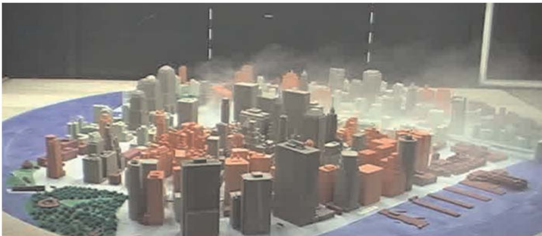
Model of World Trade Center site, Manhattan, New York City in the U.S. EPA/NOAA Fluid Modeling Facility.
