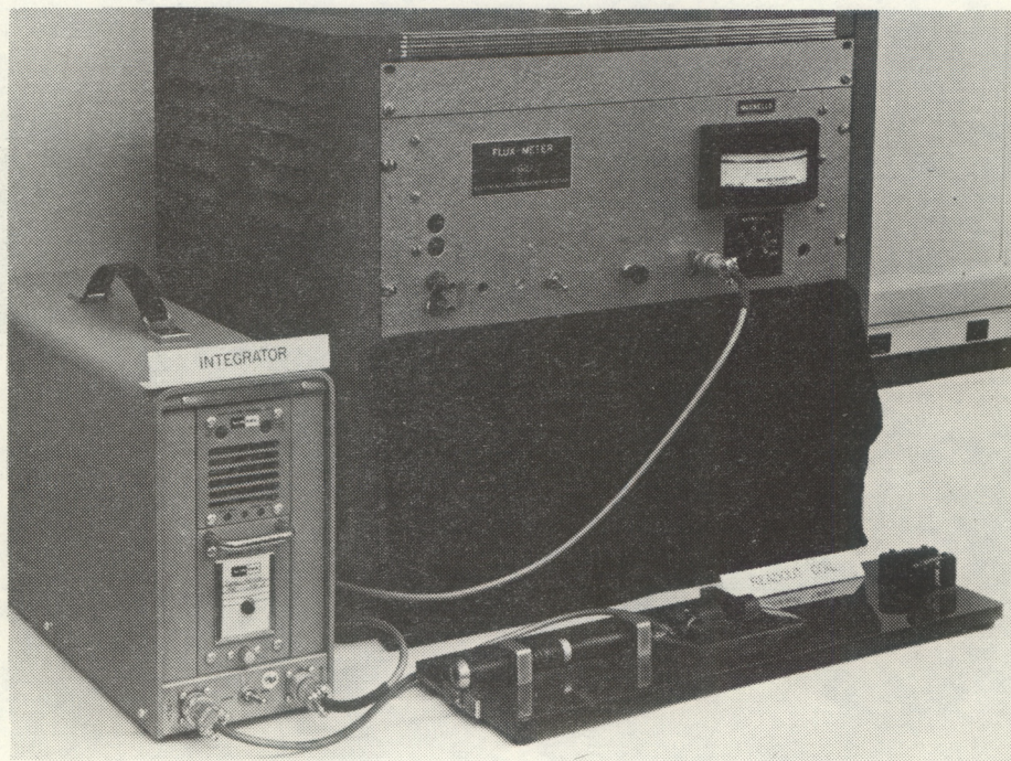
Figure 2.--Readout unit showing coil from which magnetized sample is propelled, integrating amplifier and fluxmeter.
