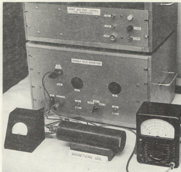
Figure 1.--Tape magnetizing unit with magnetizing coil.
