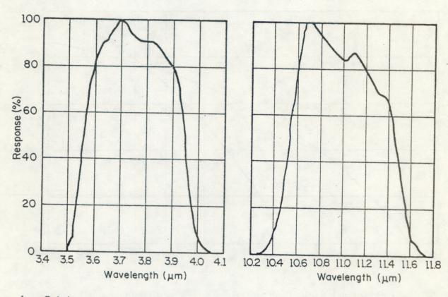
Relative spectral response functions (per cent) for channels 3 (left) and 4 (right) of the NOAA-6 satellite (from Kidwell, 1979).
