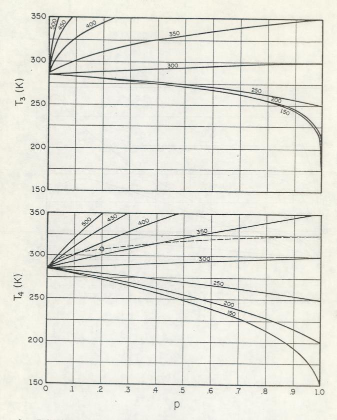
3.  $T_3$  (top) and  $T_4$  (bottom) vs. p for increasing values of  $T_t$ , for  $T_b = 285$  K. The dashed line in the lower graph shows the range of values permissible when  $T_3 = 325$ .
