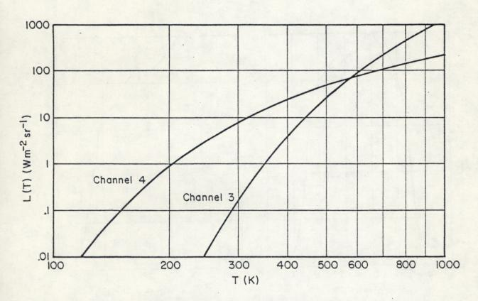
2. NOAA-6 radiances for channels 3 and 4  $\nu$ s. temperature, as calculated by eq. (1) with the spectral response functions in figure 1.
