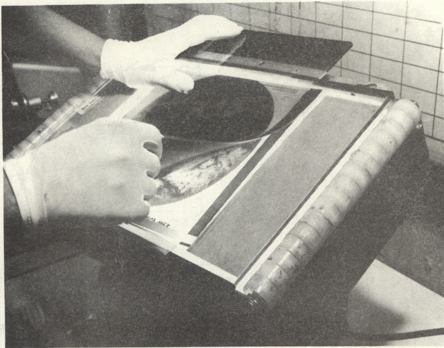
Figure 4.--Photo technician alining picture negatives with the aid of a pin registry jig and light table.
