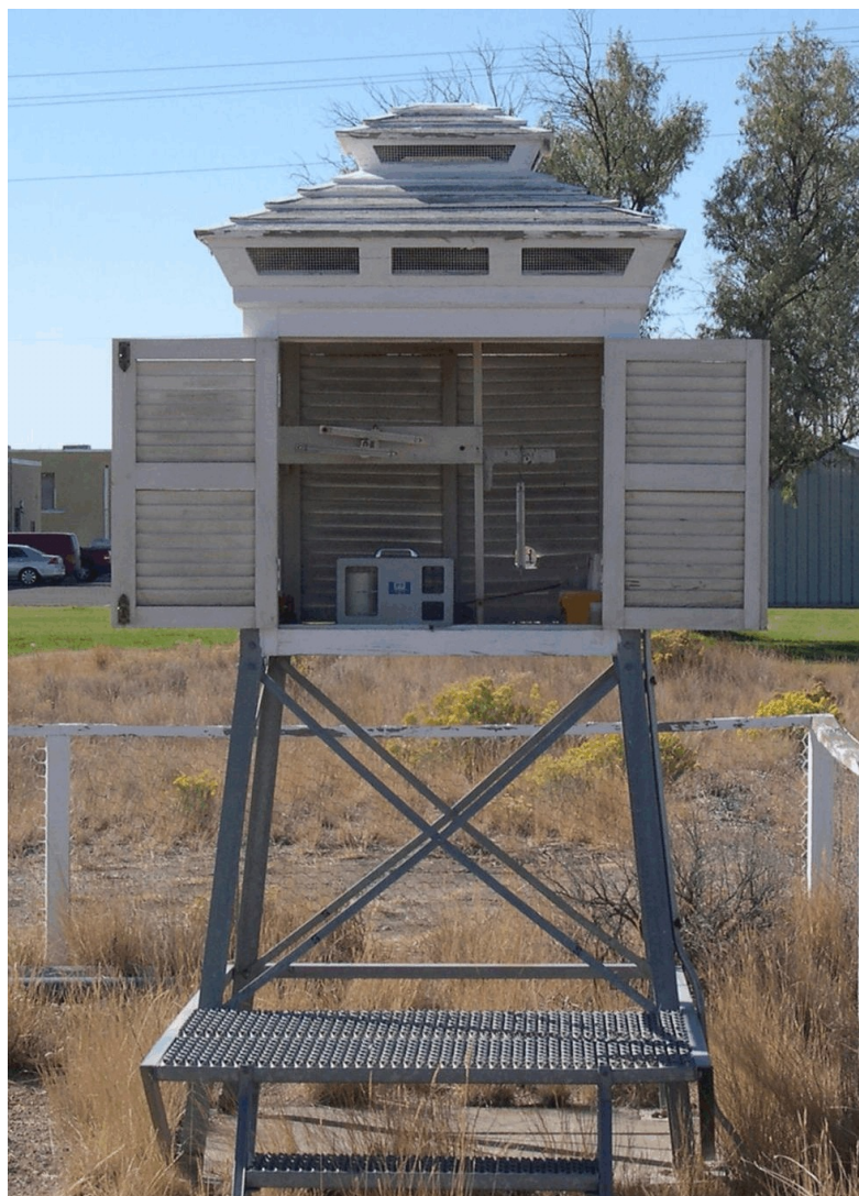
Figure 8. CFA thermoscreen is the longest and most complete air temperature and precipitation dataset at the INL.
