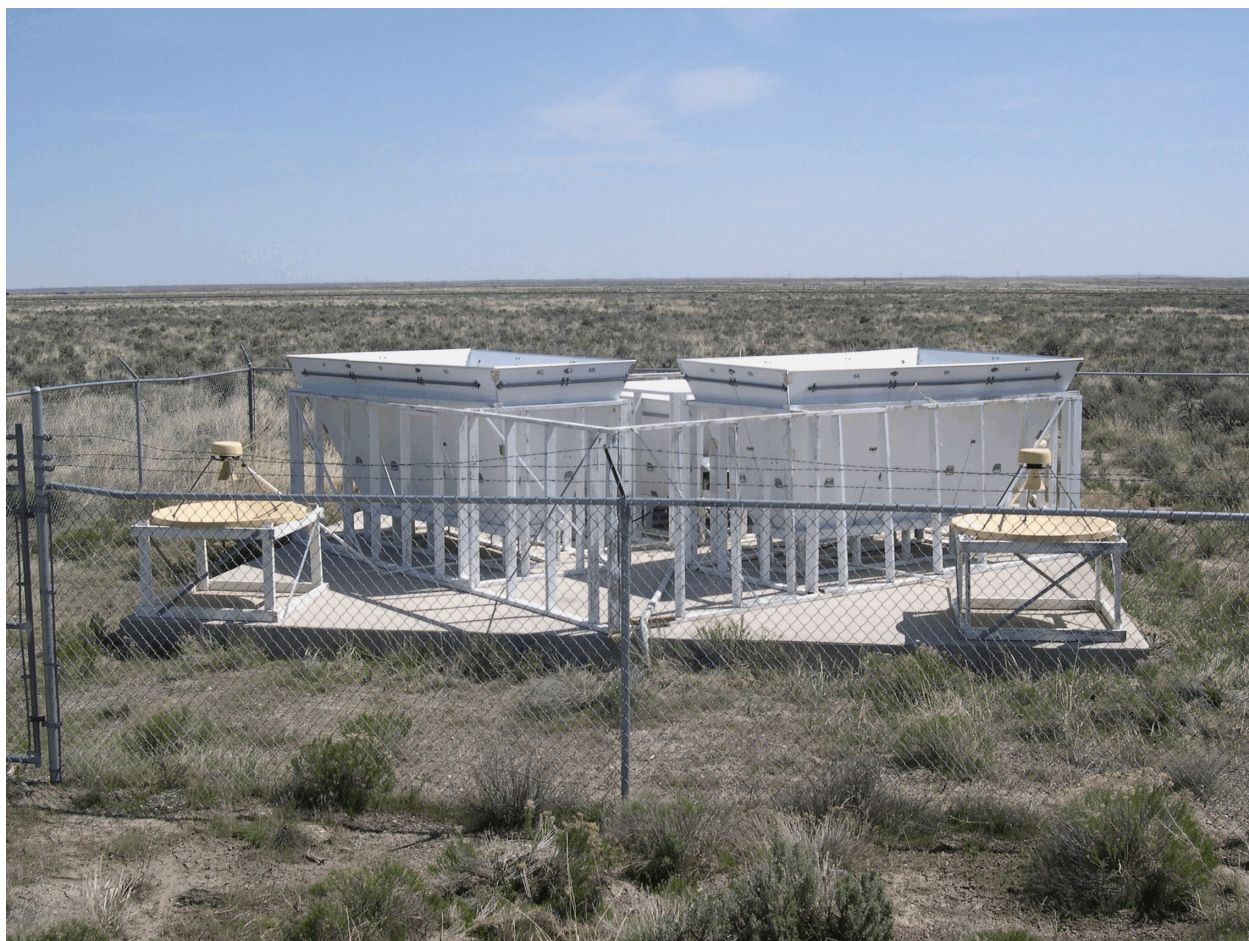
Figure 9. Radar wind profiler and RASS located near Grid 3, just north of INTEC.
