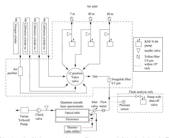
**Figure 4.** Schematic overview of the instrument setup for tower profile measurements at the Lutjewad monitoring station. The pressure sensor and pump with shut-off valve were added for flask measurements only (see Sect. 2.6).
