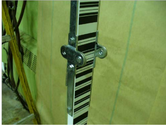
Figure 5 - Close-up of the Trimble LD23 bracket and latch system.
