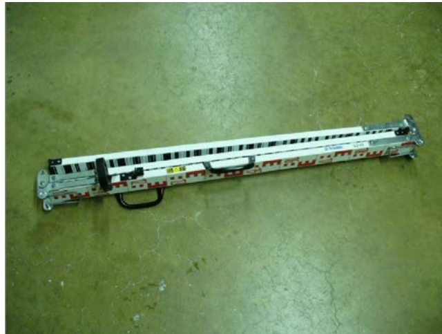
Figure 3 - Trimble LD23 folding multi-piece level staff.
