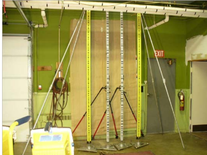
Figure 6 - Trimble level staffs setup for lab environment measurements.
