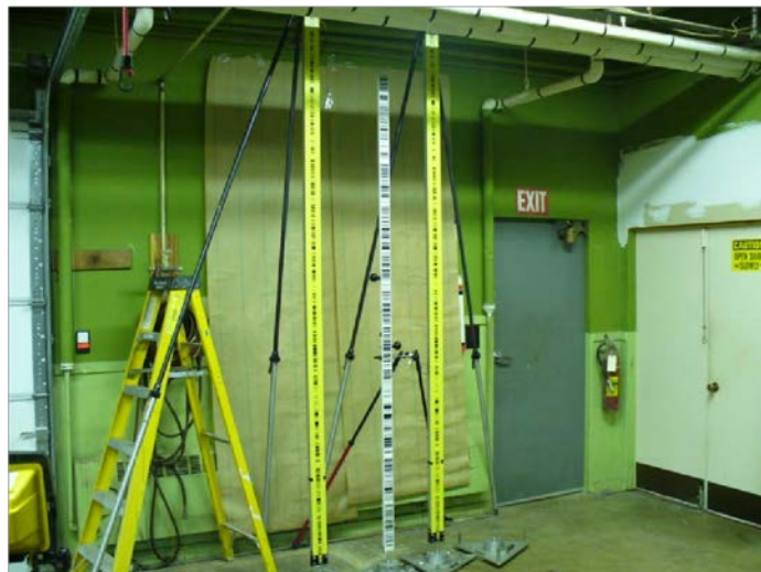
Figure 7 - Leica level staffs setup for lab environment measurements
