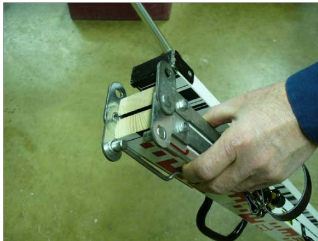
Figure 4 - Close-up of the Trimble LD23 wood core.
