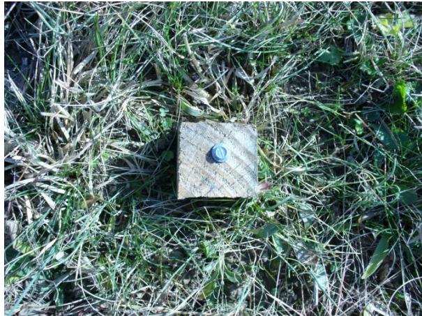
Figure 11 – Wooden hub (HUB1) with screw-head turning point.
