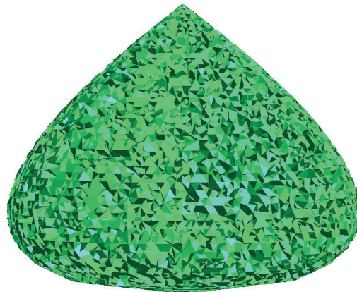
Figure 7. BRM model of a conical graupel particle used for scattering calculations.
