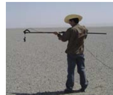
Figure 2. Portable instruments measuring the directional reflectance.
