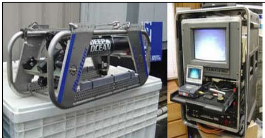
Figure 1: TOAD's underwater platform (left) and video recording system (right)
