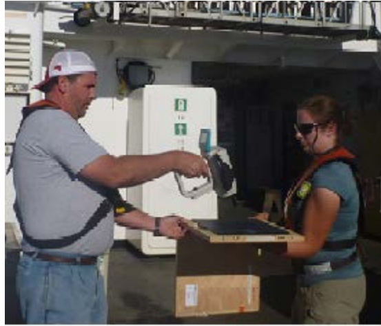
Figure 8. Science team measuring the NIST blue tile with a handheld radiometer.
