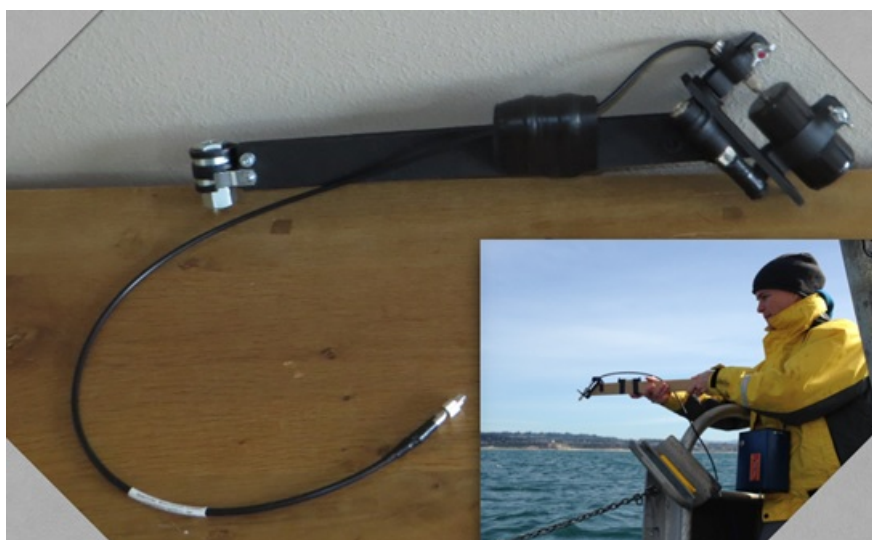
Figure 32. Mounting bracket and sensor head for Spectral Evolution spectrometer; (inset) typical operation of above water radiometer.
