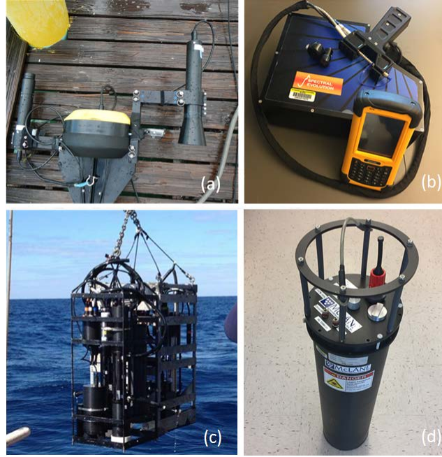
Figure 27. Instruments used on the 2016 VIIRS cruise: (a) Radiometer incorporating the Skylight-Blocked Apparatus (RISBA), (b) Spectral Evolution SR-1901, (c) IOP package including ac-s and BB9, and (d) Imaging Flow Cytobot.
