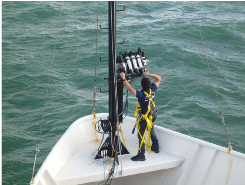
Figure 15. HyperSAS-POL on the mast at the bow of the ship.
