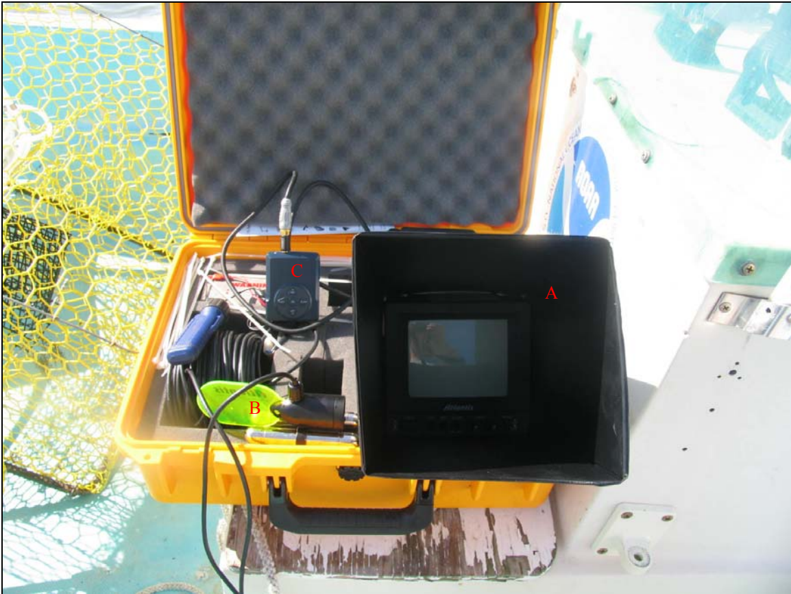
Figure 2. Atlantis Underwater Viewing System used to capture video of buoy line movements (A= on board monitor; B= underwater camera; C= DPC-1000 digital video recorder).
