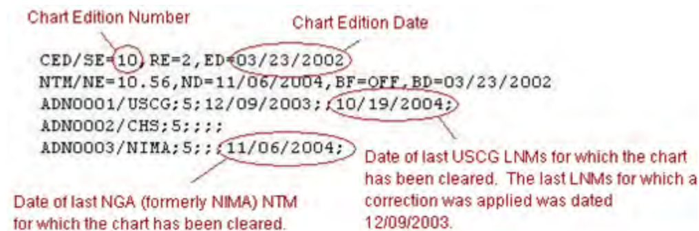
Figure 4.23: Section of a *.KAP file (opened in WordPad) identifying chart edition and corrections that have been applied to the digital file. Note: CHS does not issue corrections for this chart area, so no cleared date is listed.
