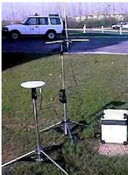
Figure 3.2: DGPS Reference Station
