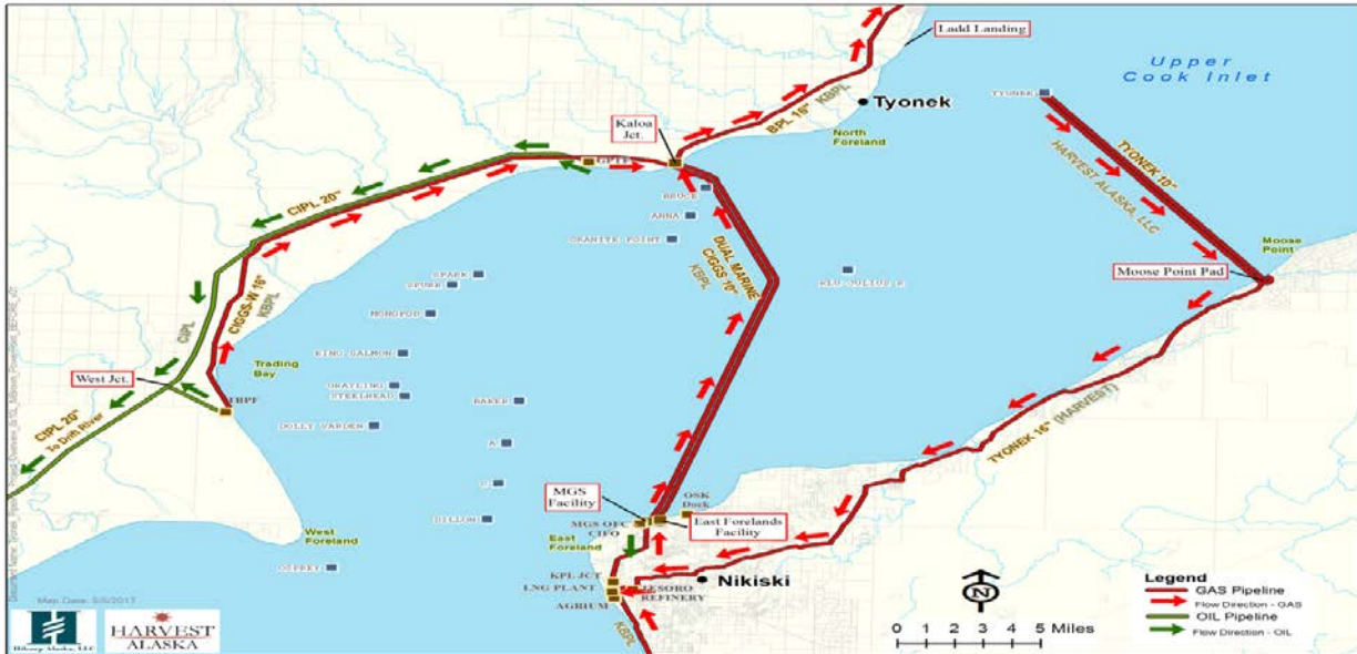
Figure 2. Current Harvest LLC oil and gas flow.
