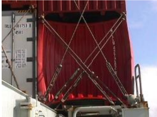
Figure 7. Lashing rods tightened by turnbuckles are attached by hand by longshoremen to help secure loads. (This container was damaged by a bow-slammng wave). Figure from Koning 2009.
