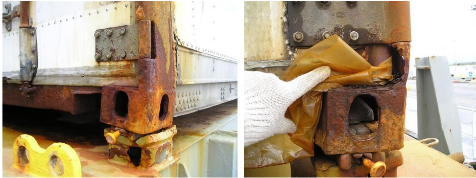
Figure 8. Container corner posts and fittings in unsatisfactory condition. Figures from AIMU 2008.
