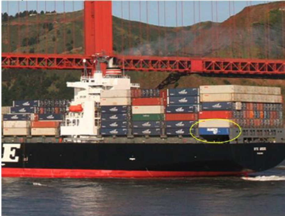
Figure 19. The NYK Argus leaving San Francisco Bay, with an instrumented MARIN container on the bottom tier to help monitor forces while underway. Photo credit: MARIN 2009.
