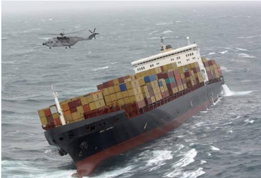
Figure 6. The MSC Napoli , which broke apart in January 2007 in the English Channel. MAIB investigation determined that 20% of the containers were overweight. Photo from AIMU 2008.
